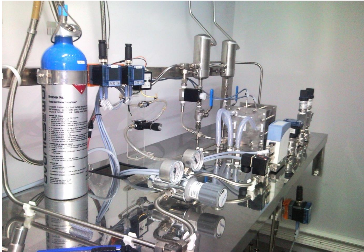
Figure 3. Hydrogen-Based Energy Source Consisting of Hydrogen Storage, Fuel Cell, Valves, and Measurement Equipment
